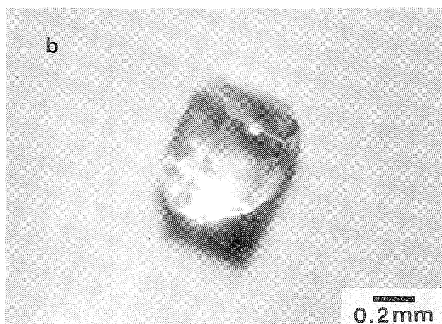
Fig. 3. Photomicrographs of calcite crystals grown in 3 \text{ mol kg}^{-1} NaCl solution at 500^\circ\text{C} and 100 \text{ MPa} for 10 d.
